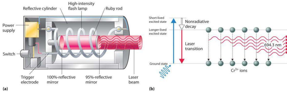
(a) This cutaway view of a ruby laser shows the ruby rod, the flash lamp used to excite the Cr<sup>3+</sup> ions in the ruby, and the totally and partially reflective mirrors. (b) This schematic drawing illustrates how light from the flash lamp excites the Cr<sup>3+</sup> ions to a short-lived excited state, which is followed by decay to a longer-lived excited state that is responsible for the stimulated in-phase emission of light by the laser.
