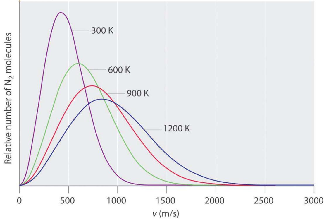
*Increasing the temperature increases both the most probable speed (given at the peak of the curve) and the width of the curve.*
