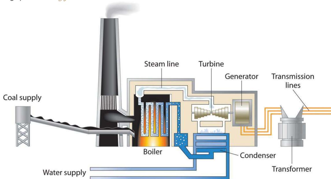
*A coal-powered electric power plant uses the combustion of coal to produce steam, which drives a turbine to produce electricity.*
