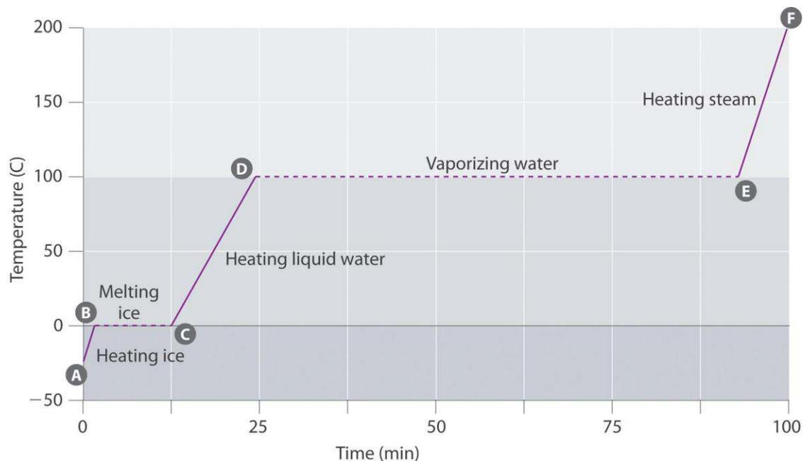
*This plot of temperature shows what happens to a 75 g sample of ice initially at 1 atm and  $-23^{\circ}\text{C}$  as heat is added at a constant rate: A–B: heating solid ice; B–C: melting ice; C–D: heating liquid water; D–E: vaporizing water; E–F: heating steam.*
