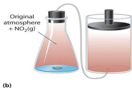
(a) Initially, the system (a copper penny and concentrated nitric acid) is at atmospheric pressure. (b) When the penny is added to the nitric acid, the volume of  $\text{NO}_2$  gas that is formed causes the piston to move upward to maintain the system at atmospheric pressure. In doing so, the system is performing work on its surroundings.
