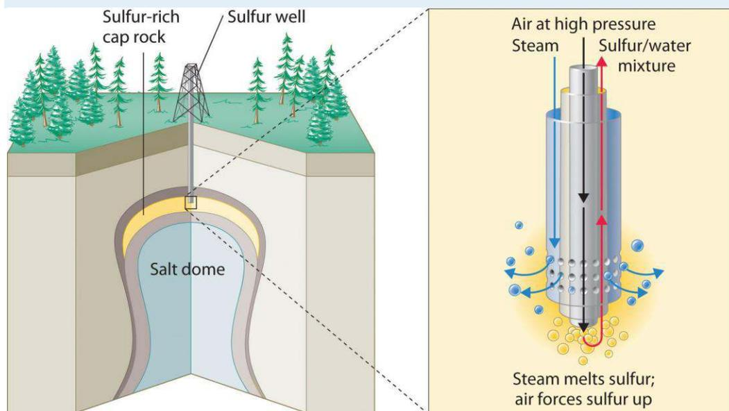
*In the Frasch process for extracting sulfur, very hot water at high pressure is injected into the sulfur-containing rock layer to melt the sulfur. The resulting mixture of liquid sulfur and hot water is forced up to the surface by compressed air.*
