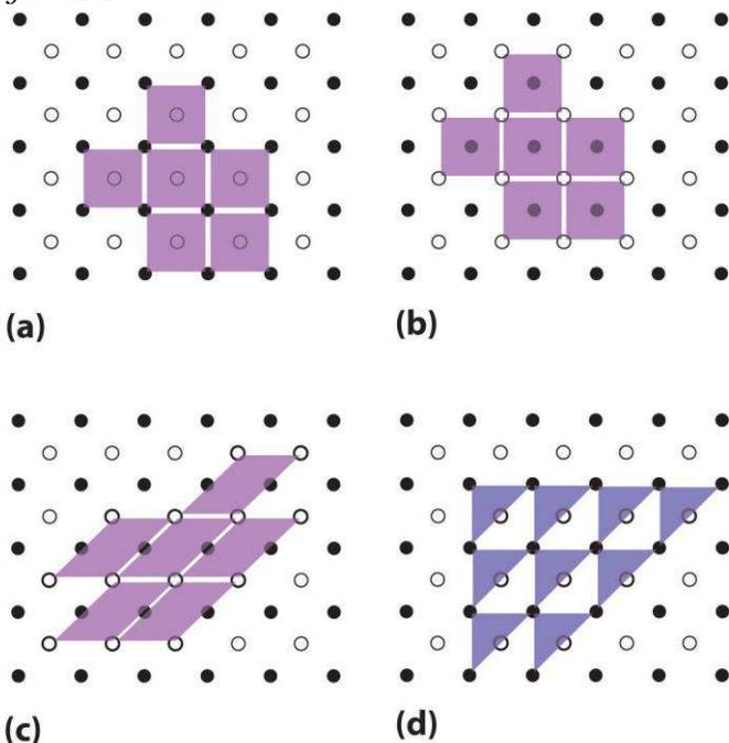
(a–c) Three two-dimensional lattices illustrate the possible choices of the unit cell. The unit cells differ in their relative locations or orientations within the lattice, but they are all valid choices because repeating them in any direction fills the overall pattern of dots. (d) The triangle is not a valid unit cell because repeating it in space fills only half of the space in the pattern.
