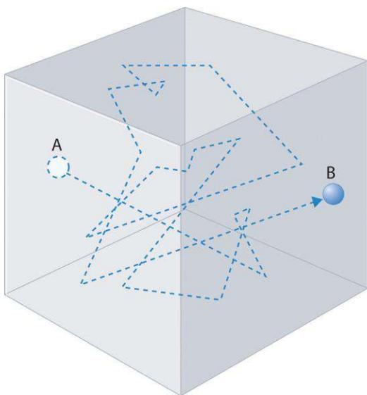
The frequent changes in direction are the result of collisions with other gas molecules and with the walls of the container.
