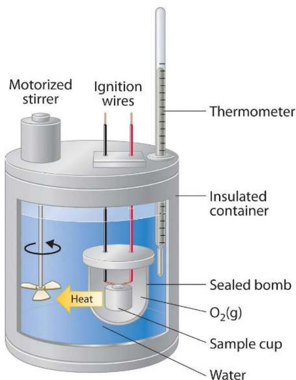
After the temperature of the water in the insulated container has reached a constant value, the combustion reaction is initiated by passing an electric current through a wire embedded in the sample. Because this calorimeter operates at constant volume, the heat released is not precisely the same as the enthalpy change for the reaction.
