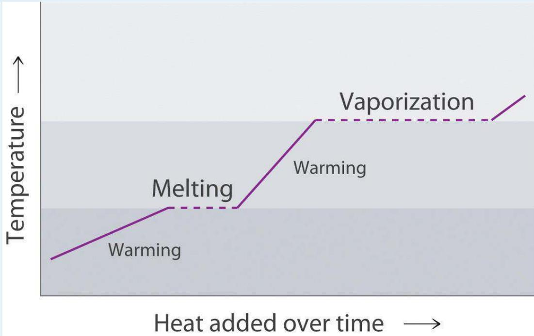
The portions of the curve with a positive slope correspond to heating a single phase, while the horizontal portions of the curve correspond to phase changes. During a phase change, the temperature of the system does not change, because the added heat is melting the solid at its melting point or evaporating the liquid at its boiling point.
