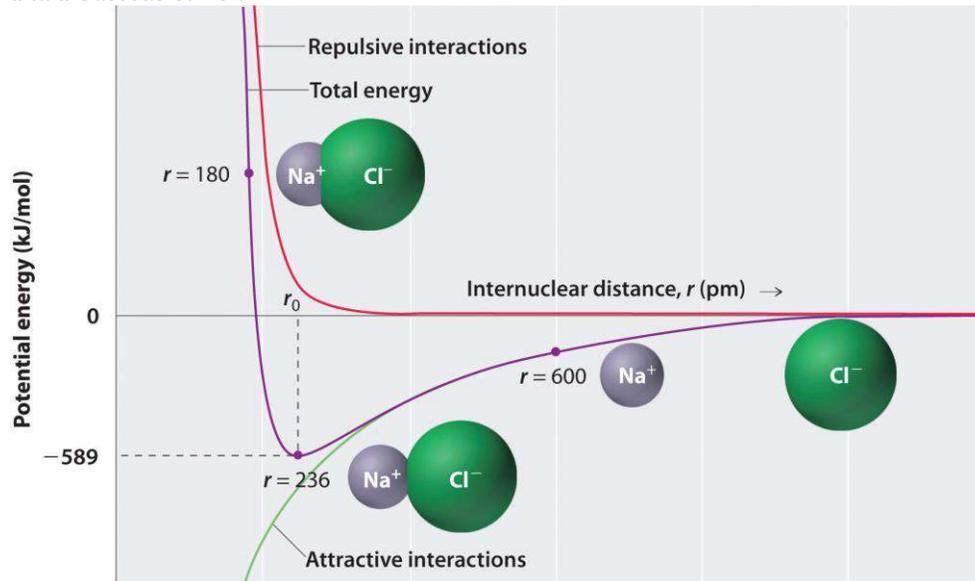
The energy of the system reaches a minimum at a particular distance ( $r_0$ ) when the attractive and repulsive interactions are balanced.
