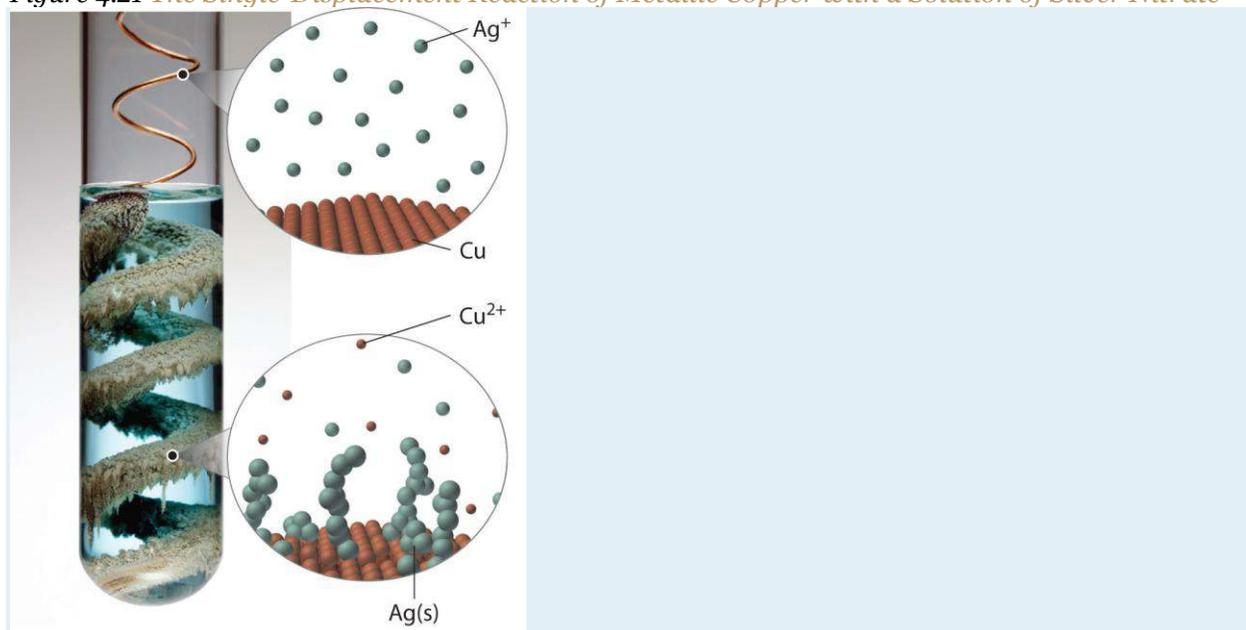
When a copper coil is placed in a solution of silver nitrate, silver ions are reduced to metallic silver on the copper surface, and some of the copper metal dissolves. Note the formation of a metallic silver precipitate on the copper coil and a blue color in the surrounding solution due to the presence of aqueous  $\text{Cu}^{2+}$  ions. (Water molecules and nitrate ions have been omitted from molecular views of the solution for clarity.)
