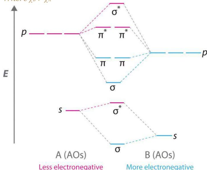
The bonding molecular orbitals are closer in energy to the atomic orbitals of the more electronegative B atom.
