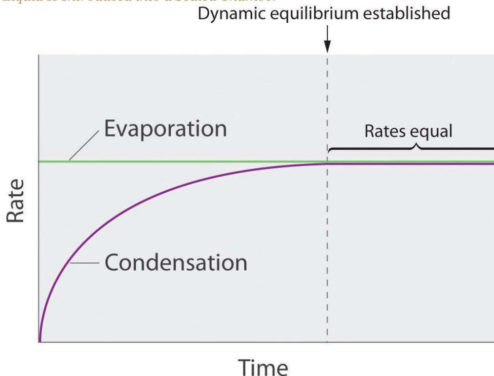
*The rate of evaporation depends only on the surface area of the liquid and is essentially constant. The rate of condensation depends on the number of molecules in the vapor phase and increases steadily until it equals the rate of evaporation.*
