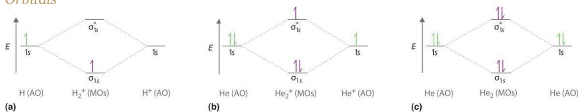
(a) The  $H_2^+$  ion, (b) the  $He_2^+$  ion, and (c) the  $He_2$  molecule are shown here.
