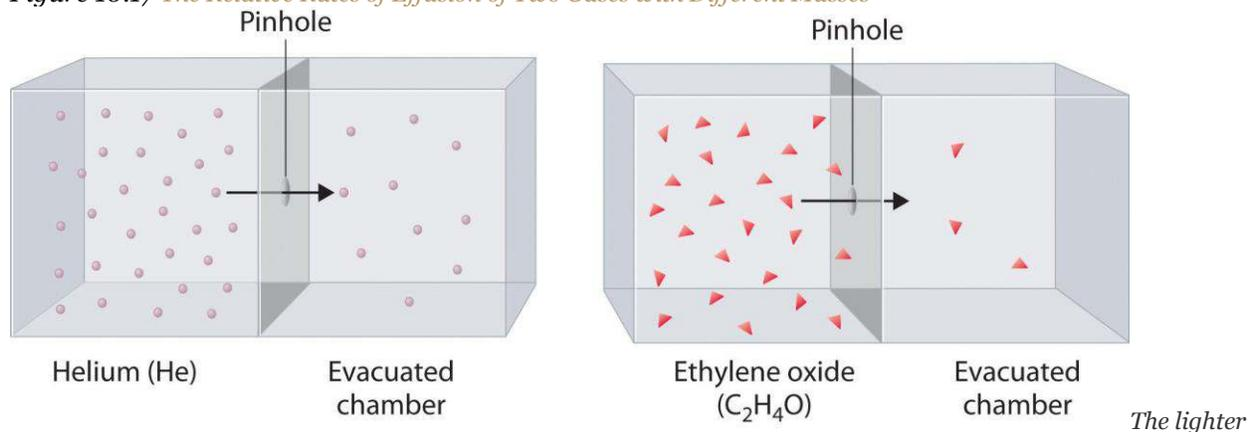
*He atoms ( $M = 4.00 \text{ g/mol}$ ) effuse through the small hole more rapidly than the heavier ethylene oxide ( $C_2H_4O$ ) molecules ( $M = 44.0 \text{ g/mol}$ ), as predicted by Graham’s law.*
