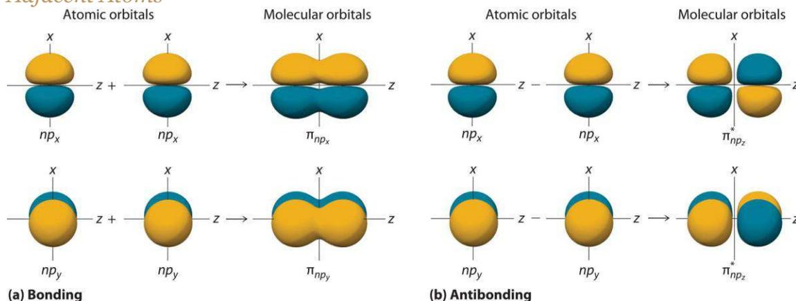
(a) Because the signs of the lobes of both the  $np_x$  and the  $np_y$  atomic orbitals on adjacent atoms are the same, in both cases the mathematical sum corresponds to a  $\pi$  (bonding) molecular orbital. (b) In contrast, in both cases, the mathematical difference corresponds to a  $\pi^*$  (antibonding) molecular orbital, with a nodal plane of zero probability density perpendicular to the internuclear axis.
