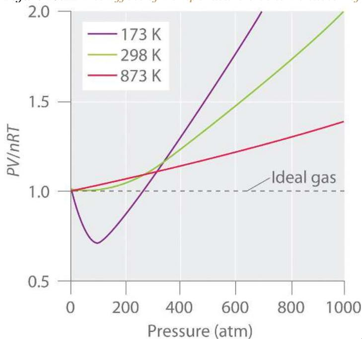
A plot of  $PV/nRT$  versus  $P$  for nitrogen gas at three temperatures shows that the approximation to ideal gas behavior becomes better as the temperature increases.
