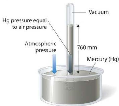
*The pressure exerted by the atmosphere on the surface of the pool of mercury supports a column of mercury in the tube that is about 760 mm tall. Because the boiling point of mercury is quite high (356.73°C), there is very little mercury vapor in the space above the mercury column.*
