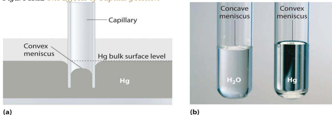
(a) This drawing illustrates the shape of the meniscus and the relative height of a mercury column when a glass capillary is put into liquid mercury. The meniscus is convex and the surface of the liquid inside the tube is lower than the level of the liquid outside the tube. (b) Because water adheres strongly to the polar surface of glass, it has a concave meniscus, whereas mercury, which does not adhere to the glass, has a convex meniscus.
