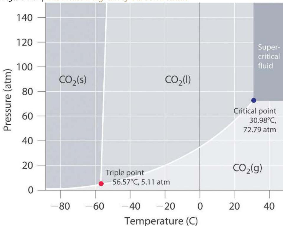
Note the critical point, the triple point, and the normal sublimation temperature in this diagram.
