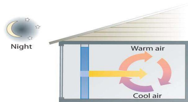
**Passive solar system.** During the day (a), sunlight is absorbed by water circulating in the water wall. At night (b), heat stored in the water wall continues to warm the air inside the house.
