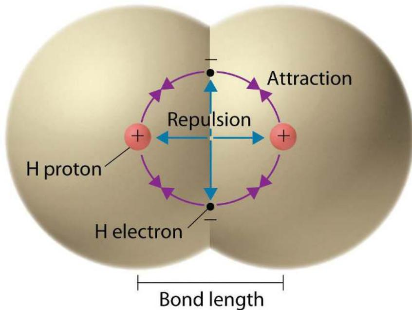
*Electron–electron and proton–proton interactions are repulsive; electron–proton interactions are attractive. At the observed bond distance, the repulsive and attractive interactions are balanced.*
