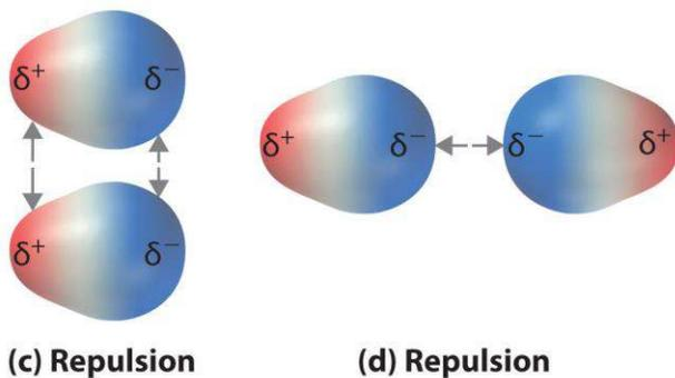
(a and b) Molecular orientations in which the positive end of one dipole ( $\delta^+$ ) is near the negative end of another ( $\delta^-$ ) (and vice versa) produce attractive interactions. (c and d) Molecular orientations that juxtapose the positive or negative ends of the dipoles on adjacent molecules produce repulsive interactions.
