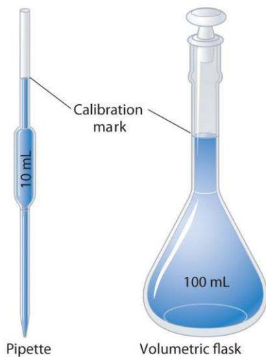
**Volumetric glassware** is used to deliver (pipette) or contain (volumetric flask) a single volume accurately when filled to the calibration mark.
