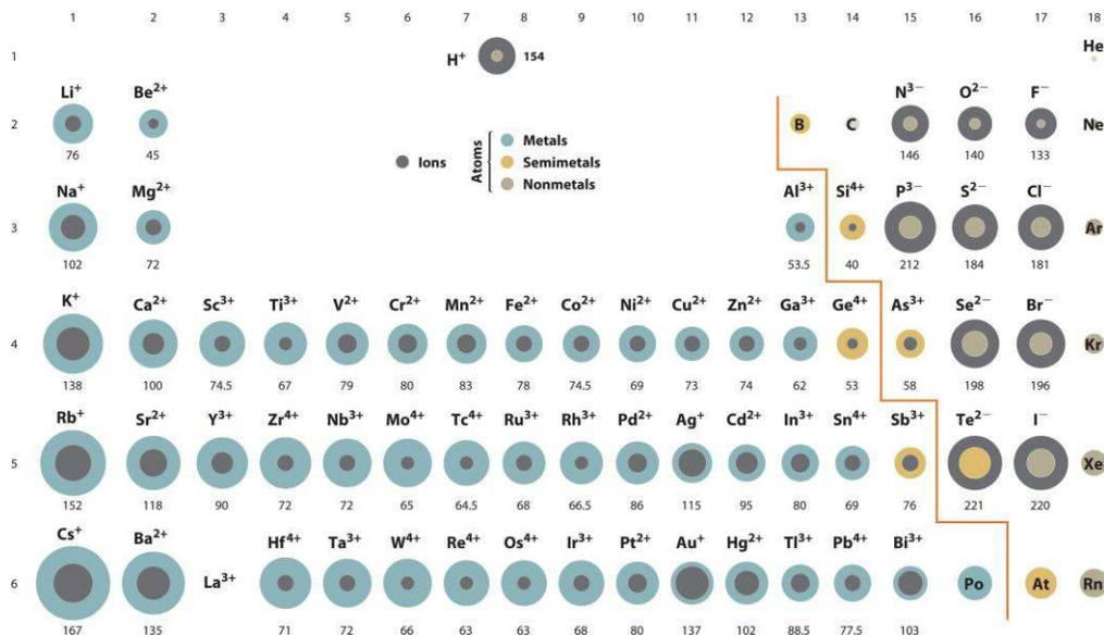
Gray circles indicate the sizes of the ions shown; colored circles indicate the sizes of the neutral atoms, previously shown in Figure 7.7 "Calculated Atomic Radii (in Picometers) of the".
