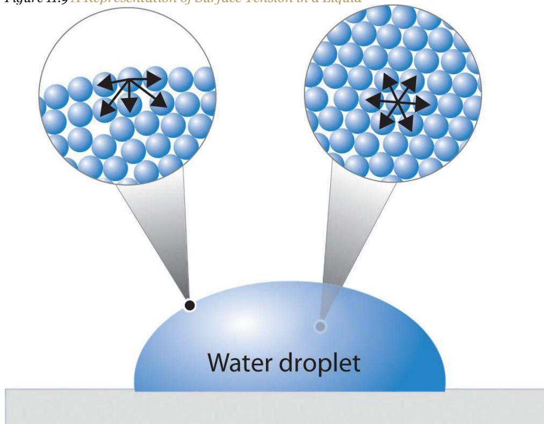
*Molecules at the surface of water experience a net attraction to other molecules in the liquid, which holds the surface of the bulk sample together. In contrast, those in the interior experience uniform attractive forces.*
