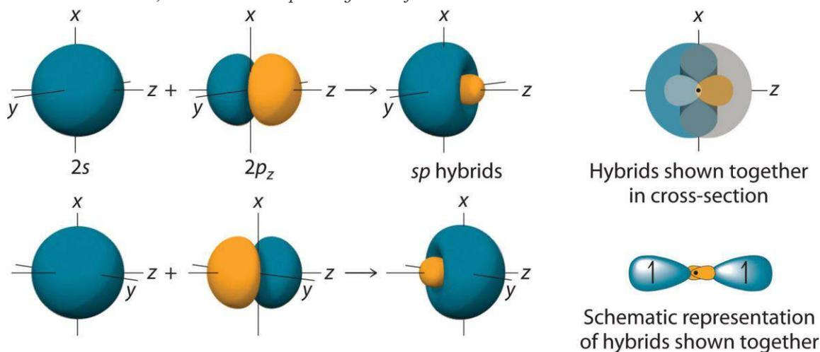
Taking the mathematical sum and difference of an  $ns$  and an  $np$  atomic orbital when  $n = 2$  gives two equivalent  $sp$  hybrid orbitals oriented at  $180^\circ$  to each other.
