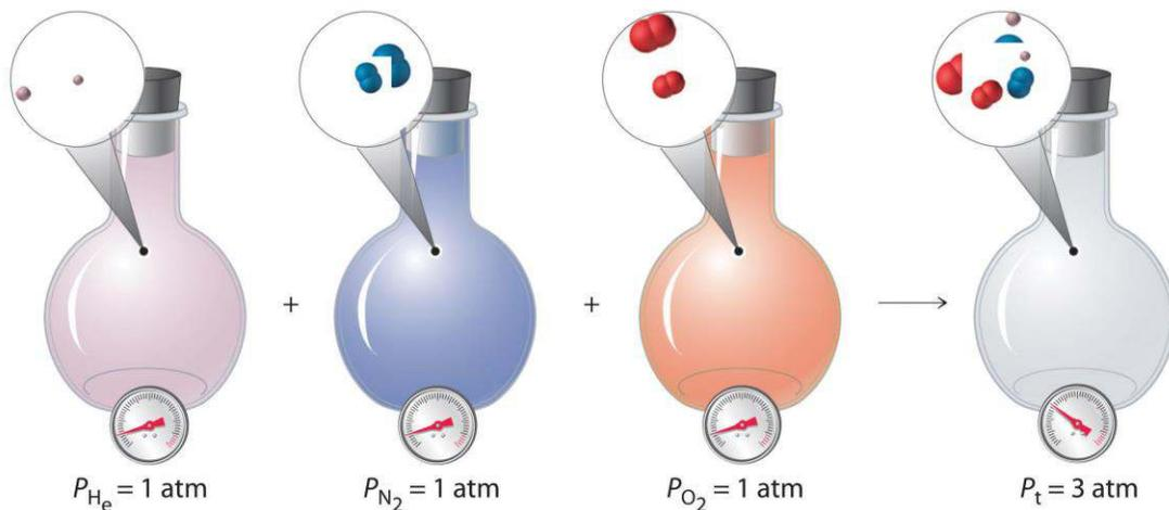
The total pressure of a mixture of gases is the sum of the partial pressures of the individual gases.
