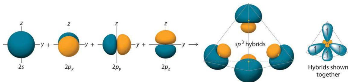
Combining one  $ns$  and three  $np$  atomic orbitals results in four  $sp^3$  hybrid orbitals oriented at  $109.5^\circ$  to one another in a tetrahedral arrangement.
