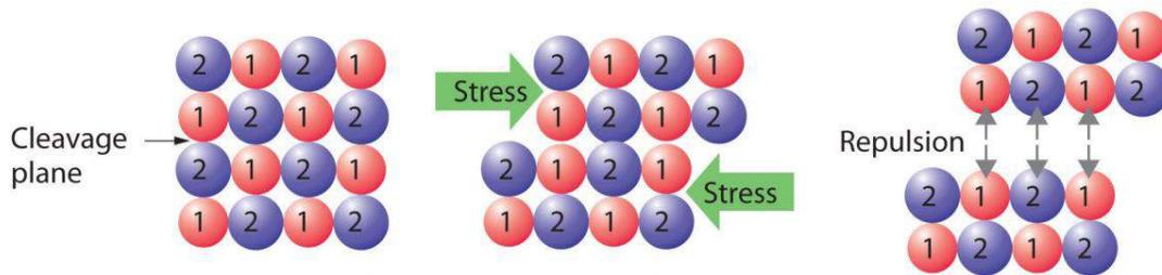
*Deformation of the ionic crystal causes one plane of atoms to slide along another. The resulting repulsive interactions between ions with like charges cause the layers to separate.*
