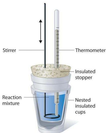
This simplified version of a constant-pressure calorimeter consists of two Styrofoam cups nested and sealed with an insulated stopper to thermally isolate the system (the solution being studied) from the surroundings (the air and the laboratory bench). Two holes in the stopper allow the use of a thermometer to measure the temperature and a stirrer to mix the reactants.
