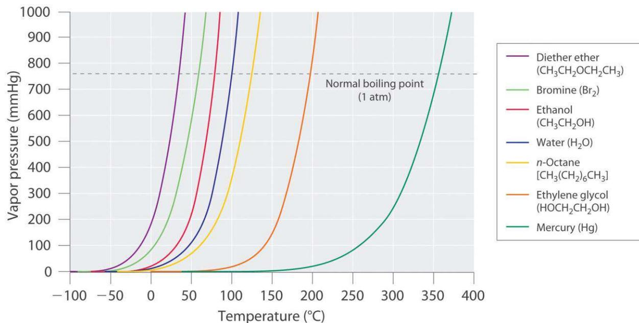
The point at which the vapor pressure curve crosses the  $P = 1 \text{ atm}$  line (dashed) is the normal boiling point of the liquid.
