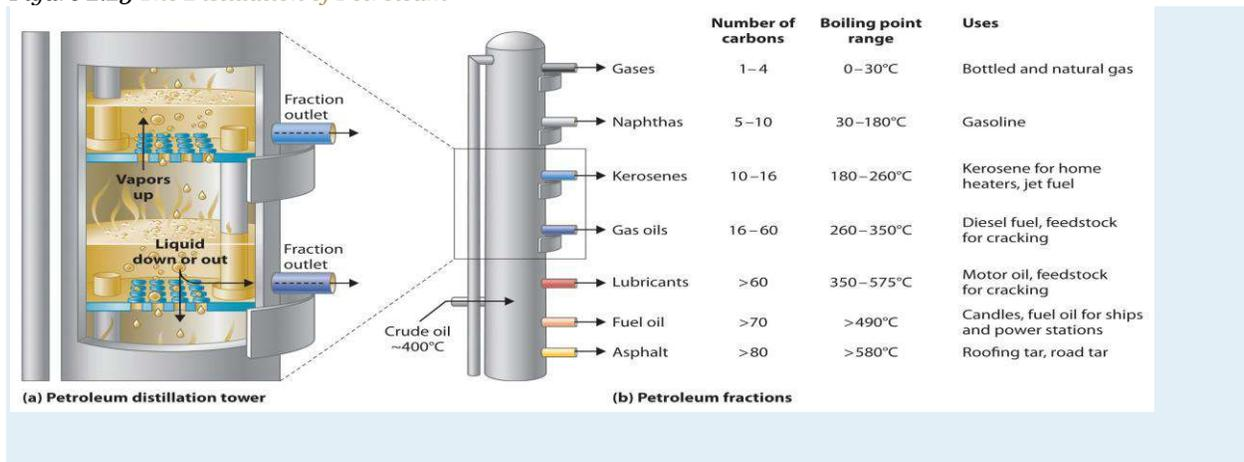
(a) This is a diagram of a distillation column used for separating petroleum fractions. (b) Petroleum fractions condense at different temperatures, depending on the number of carbon atoms in the molecules, and are drawn off from the column. The most volatile components (those with the lowest boiling points) condense at the top of the column, and the least volatile (those with the highest boiling points) condense at the bottom.
