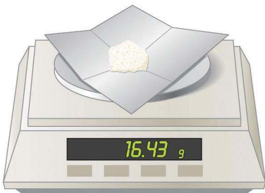
A **balance** is used to measure mass.
