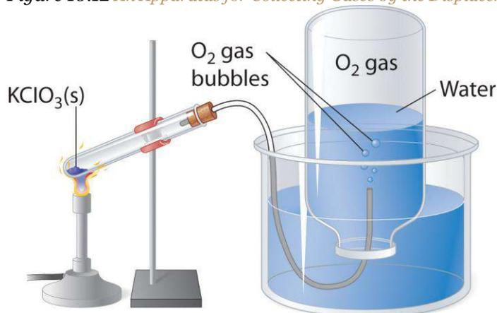
When  $KClO_3(s)$  is heated,  $O_2$  is produced according to the equation  $KClO_3(s) \rightarrow KCl(s) + 3/2 O_2(g)$ . The oxygen gas travels through the tube, bubbles up through the water, and is collected in a bottle as shown.
