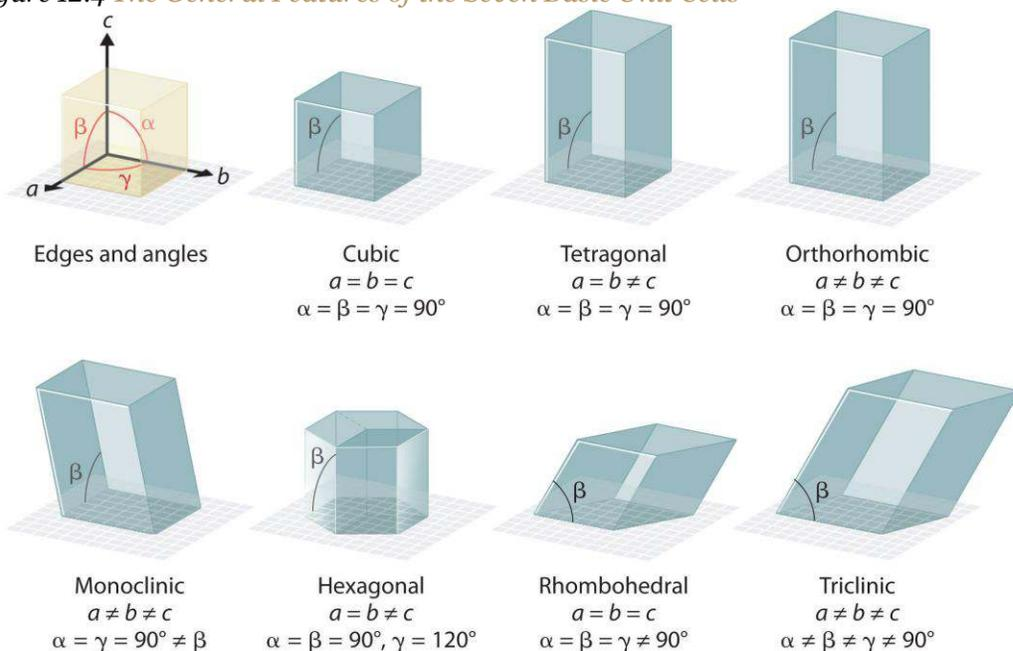
The lengths of the edges of the unit cells are indicated by  $a$ ,  $b$ , and  $c$ , and the angles are defined as follows:  $\alpha$ , the angle between  $b$  and  $c$ ;  $\beta$ , the angle between  $a$  and  $c$ ; and  $\gamma$ , the angle between  $a$  and  $b$ .
