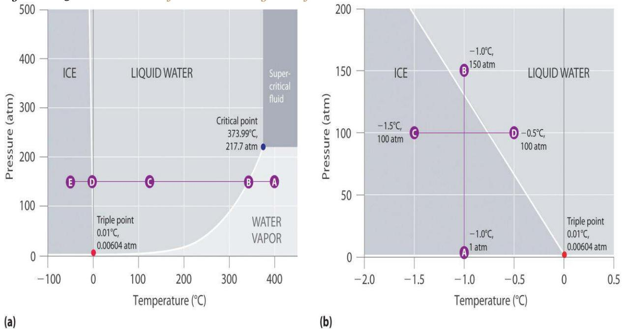
(a) In this graph with linear temperature and pressure axes, the boundary between ice and liquid water is almost vertical. (b) This graph with an expanded scale illustrates the decrease in melting point with increasing pressure. (The letters refer to points discussed in Example 10.)
