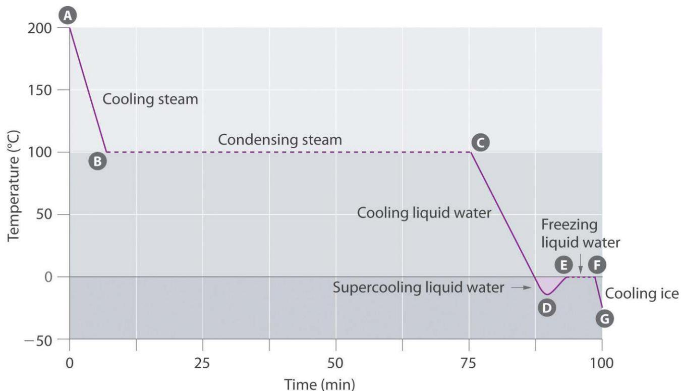
This plot of temperature shows what happens to a 75 g sample of steam initially at 1 atm and 200°C as heat is removed at a constant rate: A–B: cooling steam; B–C: condensing steam; C–D: cooling liquid water to give a supercooled liquid; D–E: warming the liquid as it begins to freeze; E–F: freezing liquid water; F–G: cooling ice.
