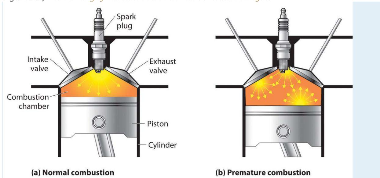
(a) Normally, fuel is ignited by the spark plug, and combustion spreads uniformly outward. (b) Gasoline with an octane rating that is too low for the engine can ignite prematurely, resulting in uneven burning that causes knocking and pinging.
