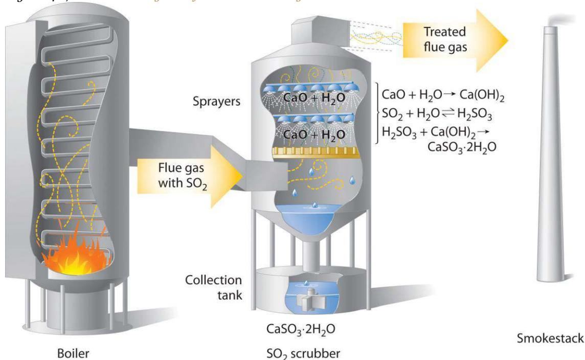
In coal-burning power plants,  $\text{SO}_2$  can be removed (“scrubbed”) from exhaust gases by its reaction with a lime ( $\text{CaO}$ ) and water spray to produce calcium sulfite dihydrate ( $\text{CaSO}_3 \cdot 2\text{H}_2\text{O}$ ). Removing  $\text{SO}_2$  from the gases prevents
