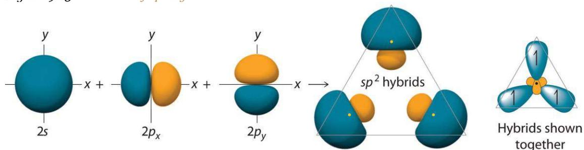
Combining one  $ns$  and two  $np$  atomic orbitals gives three equivalent  $sp^2$  hybrid orbitals in a trigonal planar arrangement; that is, oriented at  $120^\circ$  to one another.
