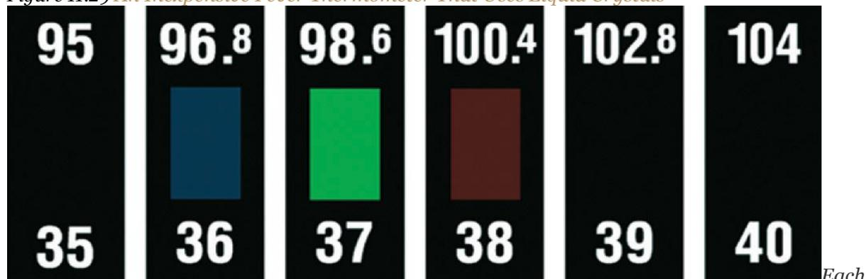
Each section contains a liquid crystal sample with a different liquid crystalline range. The section whose liquid crystalline range corresponds to the temperature of the body becomes translucent (here shown in green), indicating the temperature.
