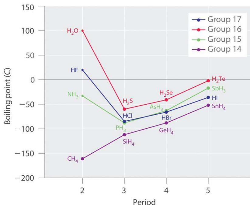
These plots of the boiling points of the covalent hydrides of the elements of groups 14–17 show that the boiling points of the lightest members of each series for which hydrogen bonding is possible (HF, NH<sub>3</sub>, and H<sub>2</sub>O) are anomalously high for compounds with such low molecular masses.
