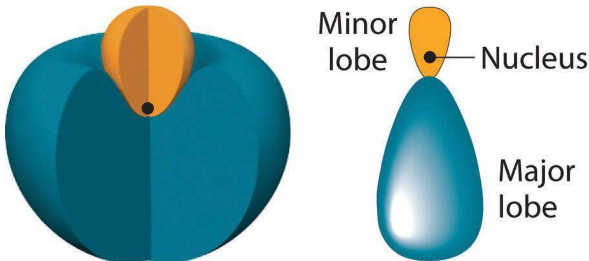
**The position of the atomic nucleus with respect to an  $sp$  hybrid orbital.** The nucleus is actually located slightly inside the minor lobe, not at the node separating the major and minor lobes.
