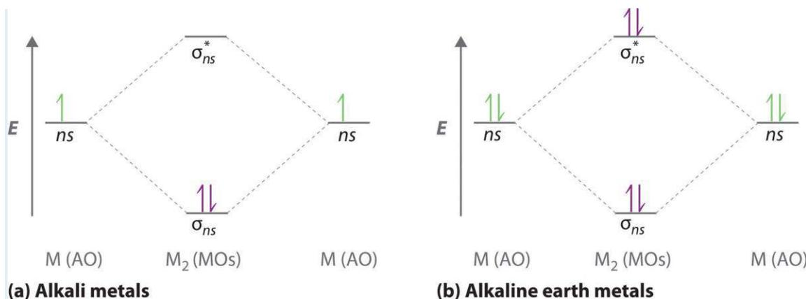
(a) For alkali metal diatomic molecules, the two valence electrons are enough to fill the  $\sigma_{ns}$  (bonding) level, giving a bond order of 1. (b) For alkaline earth metal diatomic molecules, the four valence electrons fill both the  $\sigma_{ns}$  (bonding) and the (nonbonding) levels, leading to a predicted bond order of 0.
